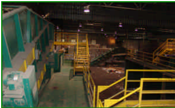
The machine on the left is called a disc screener
